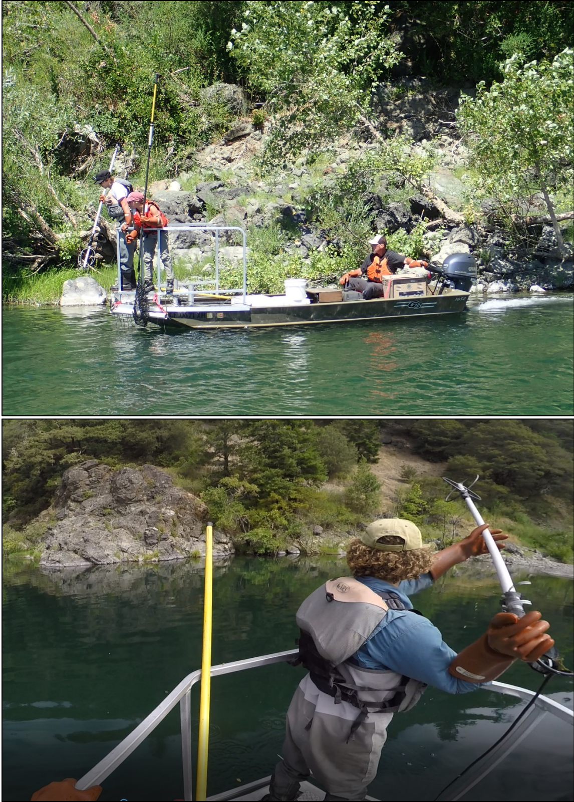
Figure 5. Jon boat equipped with a throw anode set-up (top) and throw anode being deployed (bottom).
