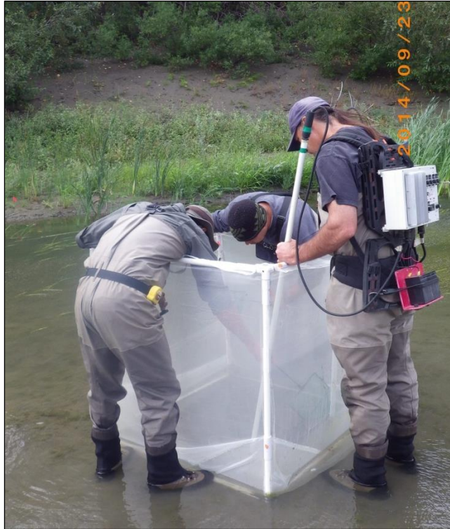
Figure 2-4. The 1-m 3 netted frame used for sampling ammocoetes in selected sample quadrats at index survey sites.
