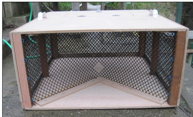
Figure 4. Plywood box trap designed to capture upstream migrating adult Pacific lampreys at the HFAC weir on Freshwater Creek during lower stream flows (Photo by C. Anderson).
